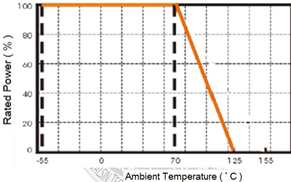
Fig.1 Maximum dissipation in percentage of rated power
