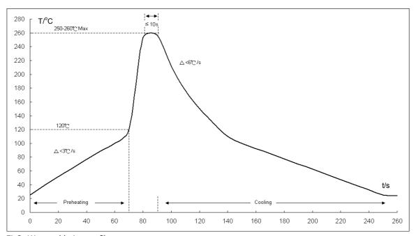
Fig2: Wave soldering profile
