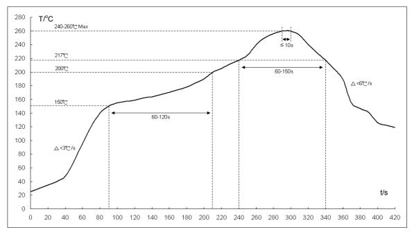
Fig1: Reflow soldering profile for lead-free solder (SnAgCu)
